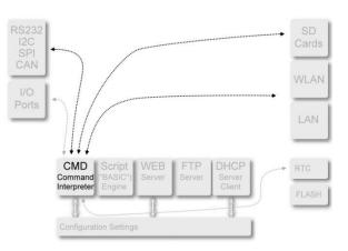
typing in commands and by reading the answer on the terminal. The command interface is available on all physical interfaces (CAN, SPI, I2C, ...).
